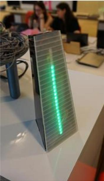
**Figure 1.** The TangiPlan prototype consists of a set of objects that represent routine morning tasks, which are spread around the house in locations relevant to a target task. Each object communicates with a central server and offers a visual representation of the time allocated to the corresponding task. Each object also gives real-time feedback of the gradual count-down of time left to complete the task.
