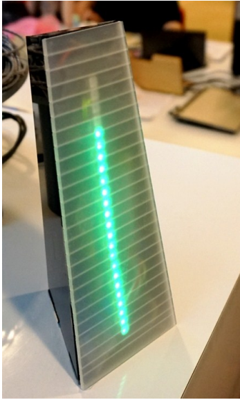
Figure 1. The TangiPlan prototype consists of a set of objects that represent routine morning tasks. The objects are placed around the house in locations relevant to a target task. Each object communicates with a central server and offers a visual representation of the time allocated to the corresponding task. Each object also gives real-time feedback of the gradual count-down of time left to complete the task.
