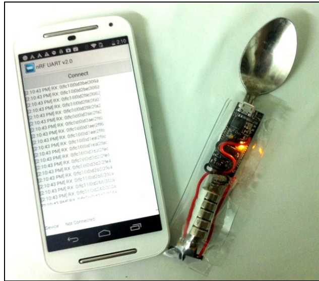
Figure 2. Initial prototype of SenSpoon: a standard spoon augmented with the IMUduino BTLE board to monitor various biomechanical variables during self-feeding. Data is streamed via Bluetooth to a smartphone.
