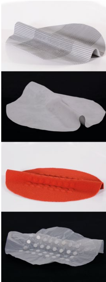
Figure 1: Material experimentation. From the top: fluted foam, Tyvek, plastic and textile. Each with 4 magnets. Some include acrylic disks added to accentuate the form.
