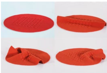
Figure 4: Actuated material movement in 2D forming a 3D shape in the material layer.
